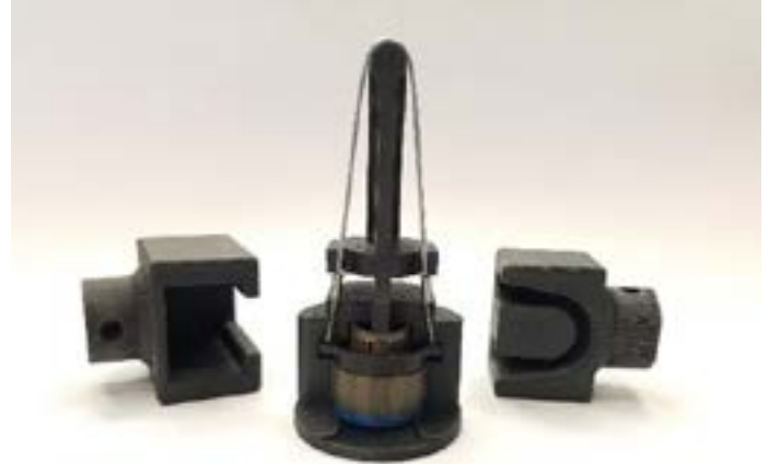
PROTOTYPE/PRODUCTION TOOLING - 3D PRINTED NYLON 12 CF: DESIGNED IN SOLIDWORKS PREMIUM, PRODUCED ON THE STRATASYS FORTUS 450MC
